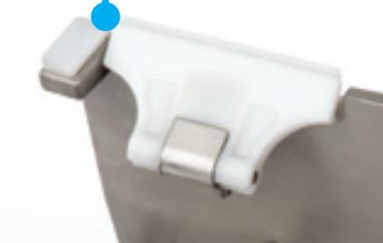
The scraping effect on the cylinder surface resulting in an extremely high heat rate efficiency as well as a high energy saving is given by the strength of the materials the scrapers are made of, their special inclination on the touch point and the specific high-thrust spring. Scrapers' material is provided with EC marking for use in food handling equipment.
